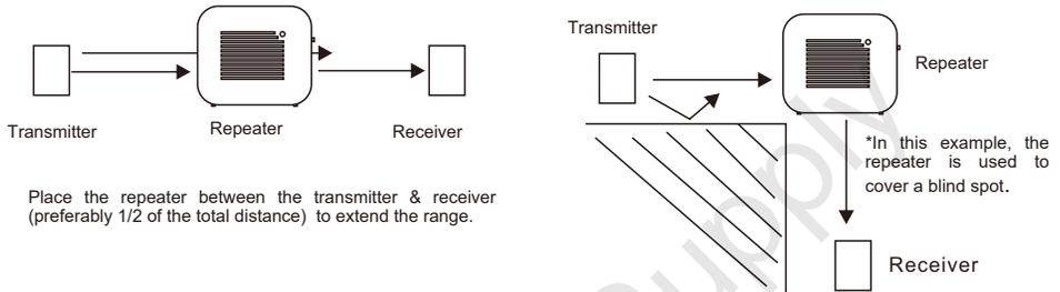
**\*\*Do not place repeaters directly in-line with one another as this could cause oscillation.**
