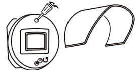
1. Remove the sun shade and the four screws holding the sensor cover in place.
