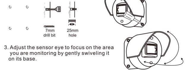
3. Adjust the sensor eye to focus on the area you are monitoring by gently swiveling it on its base.
