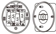
2. Inside the sensor unit is a battery compartment and the rows of switches which control the sensor settings.
