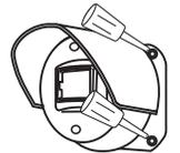
3. Adjust the sensor eye to focus on the area you are monitoring by gently swiveling it on its base.
