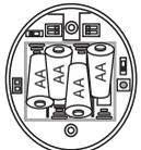
1. Remove the sensor's front cover by removing the two cover screws. Install four (4) AA batteries as indicated.
