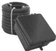
The **DCHT 4000** is a very reliable and easy-to-install driveway alarm. This transmitter operates on one 9-volt battery and has 25' of 3/8" diameter hose that lies across the drive. When a vehicle drives over the hose the sensor will send a signal back to one of our 4000 Series receivers about a mile away.\*
